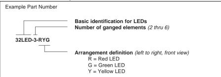
Example part number describes a stack of 3 LEDs, arranged red, yellow and green from left to right. Maximum number of stacked LEDs in this part numbering scheme is six. Contact Grayhill for stacks of more than six elements.
